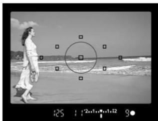
**4 Keep pressing the shutter button halfway and recompose the picture as desired.**
