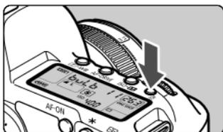
Each time you press the <☀> button, the LCD panel illumination will turn on or off (☀6). During a bulb exposure, pressing the shutter button completely will turn off the LCD panel illumination.
