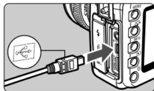
**3** Connect the camera to the printer.
