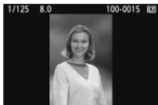
Vertical images are rotated automatically so they are displayed vertically on the camera's LCD monitor and personal computer instead of horizontally. The setting of this feature can be changed.
